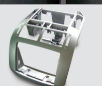
A similar injection process to die casting to produce plastic parts - employing either thermosetting or thermoplastic techniques - through the injection of molten plastic under pressure into a mould. Plastics commonly shaped by injection moulding include pvc, pe, nylon, abs and others.
